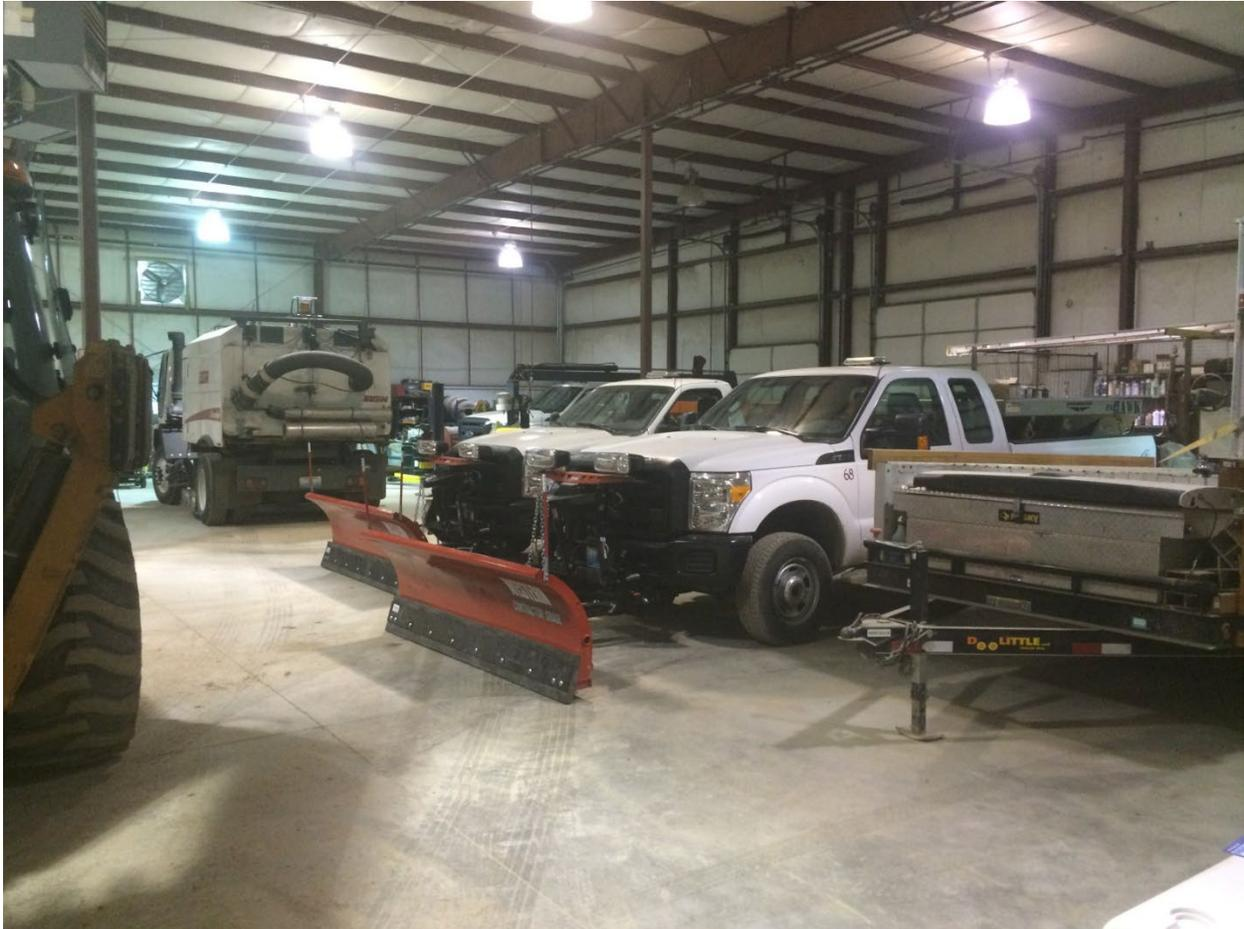
The existing truck is a 2016 model Ford F-350 medium-duty pickup truck. The truck operates during snow operations and includes a plow blade system and salt spreader. Outside of the snow plow operations, this vehicle is used regularly to haul materials, equipment, and personnel to project sites.
