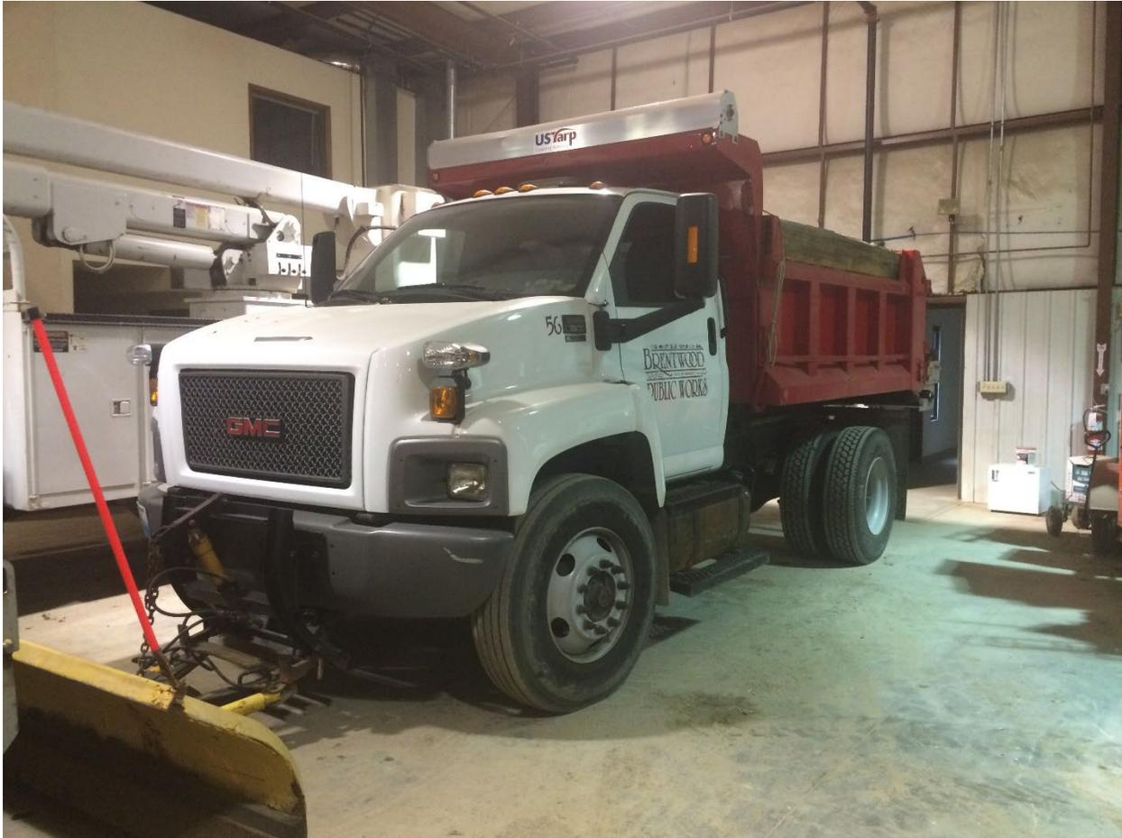
The existing truck is a 2008 model GMC C7500 heavy-duty dump truck. The truck purchase includes a plow blade system and salt spreader for operating as a plow vehicle and transporting heavy loads of materials for road projects. The vehicle model is about 18 years old which limits finding replacement parts to online brokers and not vehicle dealerships.
